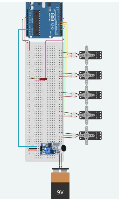
This is the TinkerCAD circuit for this project, with the 5 motors, the sound sensor, and the three LED lights.
